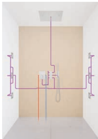
Central thermostat mixer in the shower with 3-way concealed valves Grohtherm F
